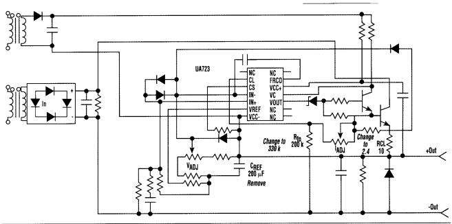
Enhancements (noted in italics) implemented into a typical power supply that uses a 723 regulator topology can boost performance. Included in the remedies are replacing the foldback resistor and the current-limit resistor and removing the reference filter capacitor.
