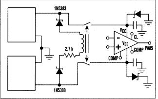
Using a voltage-sensing relay in high-voltage op amps that use two powshouldn't be used, because der supplies can cure the problem of lagging supply current caught in the foldback current limit. This occurs when one supply comes up faster than the other. The problem also arises when trying to power a group of amplifiers after successfully powering a lower-current high-voltage op amp.
